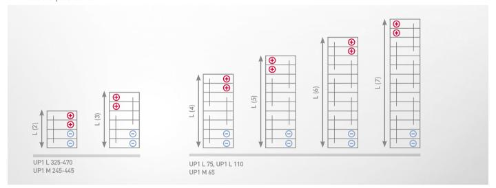
With 2-6 bolts per pole, crosswise mounted on racks
