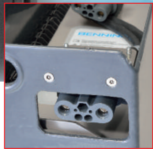
Fig. 22: An externally accessible plug-in charging connector enables fast opportunity charging without lifting the battery cover. (Option)
