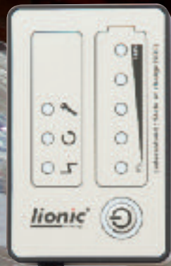
Fig. 16: External charge state and status indicator
