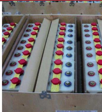
Fiber board battens are placed in between and on top of the batteries.
