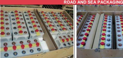
Batteries are placed in an upright positon with polystyrene filling out the crate so that no movement can take place.
