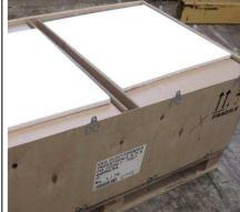
Polystyrene is placed on top of the batteries before the lid is closed.
